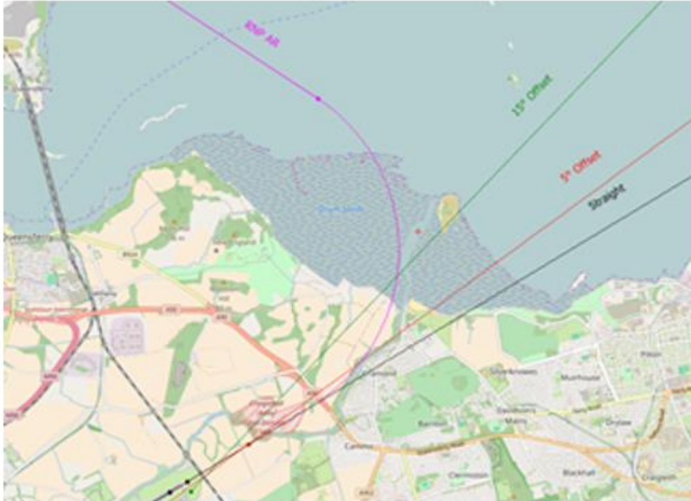
Figure 1 Example of Runway 24 Approach Routes (5° offset, a 15° offset and an RNP AR from the north)
