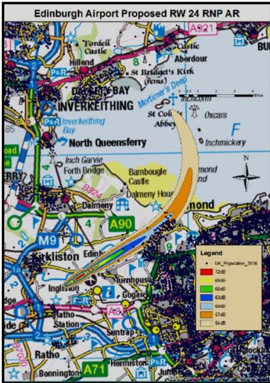
Figure 3 Noise Contours for Edinburgh Airport R24 Arrivals utilising a R24 RNP Approach
