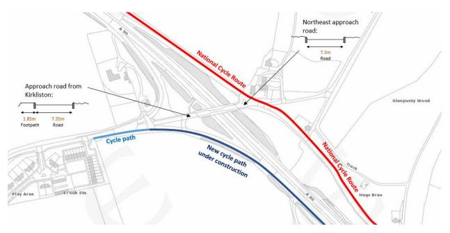
Existing cycle/pedestrian routes and approach geometries at Burnshot Bridge are shown in the image above. Slip roads allow vehicles to leave and join the A90 in both directions. A new cycle/pedestrian path is under construction which will improve the route to the Southwest side of the bridge, facilitating those cycling or walking between Edinburgh and Kirkliston.
